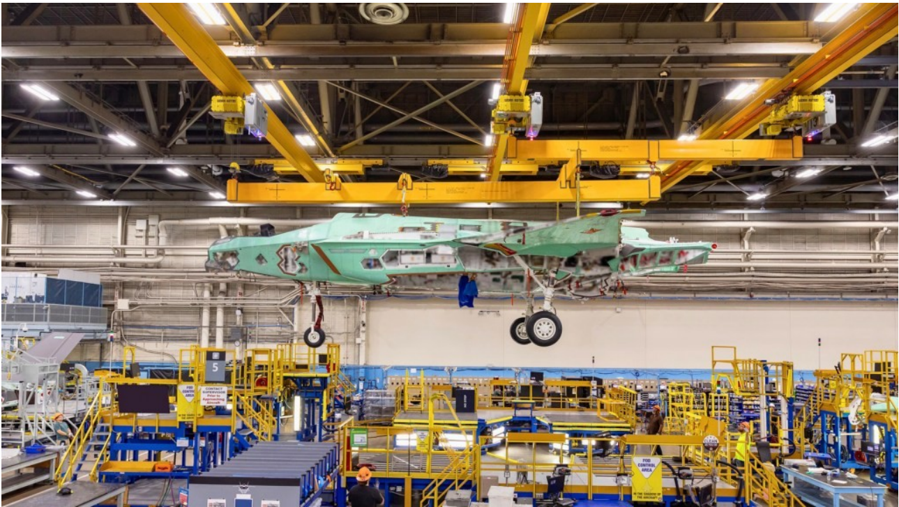
An F-35A is lifted by overhead crane to final assembly. Lockheed Martin
